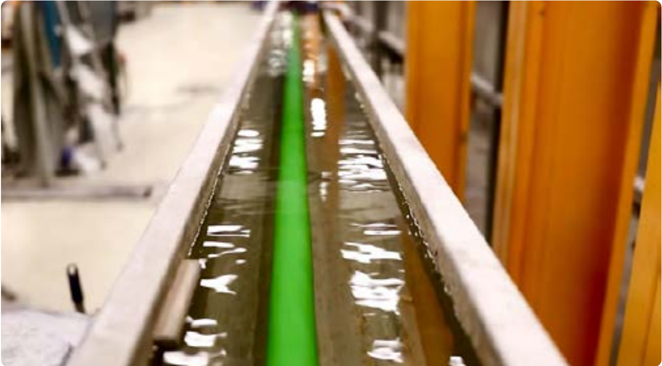
During the manufacturing process of an electrical cable, it is submerged in a water bath to dissipate the generated heat.
